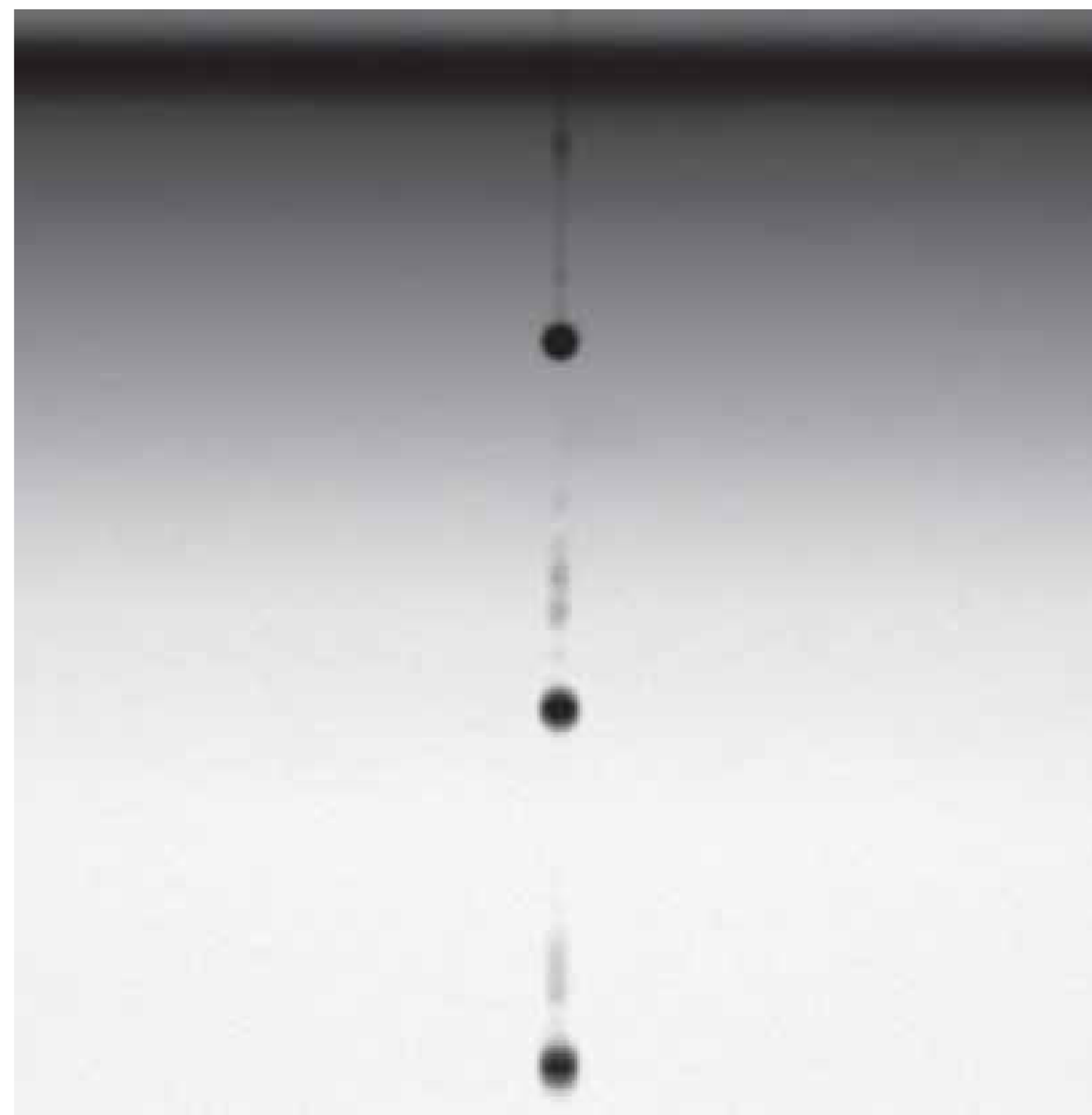
Image showing 'triple dots', 3 strobes, 3 delays per frame.
